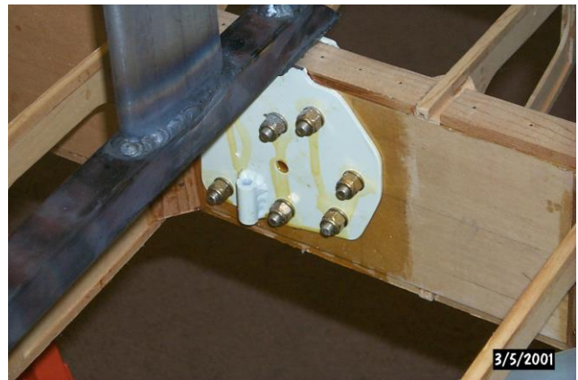
Bottom Left Wing, Front Spar, Looking forward from trailing edge of wing, I-Strut to Wing Fitting - The hole seen drilled is for the internal flying wire fittings. The bottom tube is approximately 1" long, 7/16 x 0.095, drilled and tapped for 1/4 x 28 bolt. A ring will be made with 1/4 x
