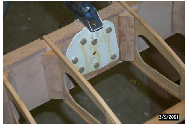
Bottom Left Wing, Front Spar, Looking aft from leading edge of wing, I-Strut to Wing Fitting - The hole seen drilled is for the internal flying wire fittings.
