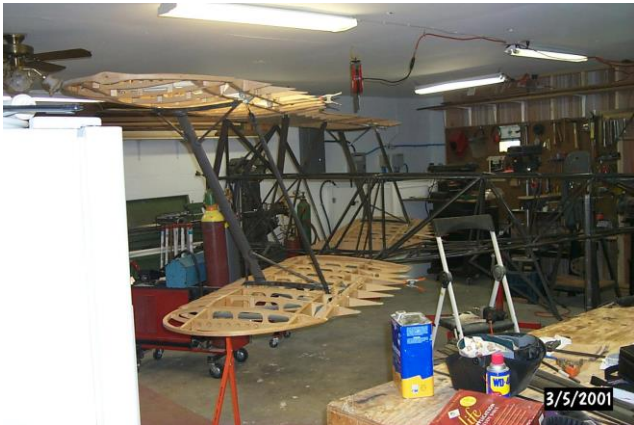
Left Upper and Lower wings, showing the I-Strut, Slave Strut, Upper and Lower ailerons, Compression tubes, aileron hangers, and aileron bellcrank.
