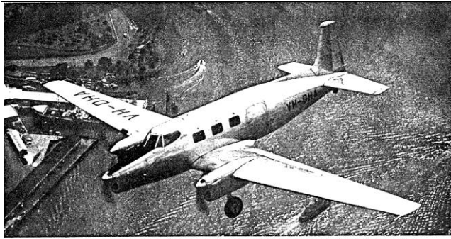
The de Havilland DHA-3 Drover Commercial Monoplane (three 140 h.p. D.H. Gipsy Major engine).
