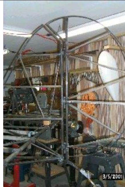
Left side view looking right of the vertical tail. Note the three hinges for the car engine stand to attach.
