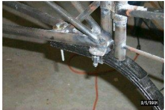
Tailwheel spring attachment
