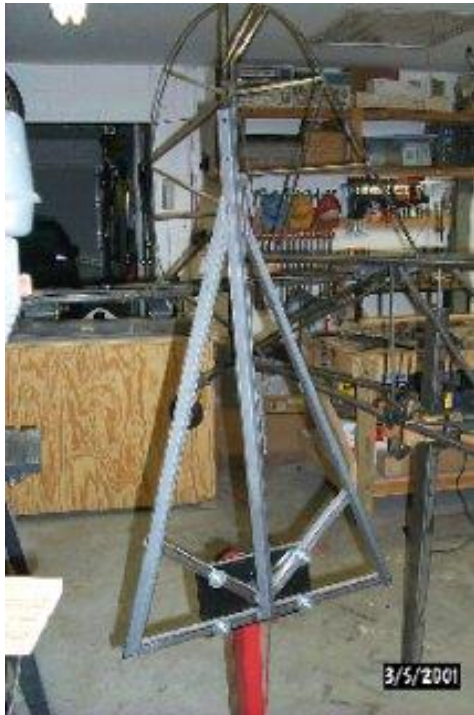
Rear car engine stand, looking from the front. The triangle portion attaches to the hinges of the vertical tail. – The two holes at the top are 3/8 inch and allow the additional bracket to bolt to this piece. Note: There are two 5/16-inch pins shown which protrude down. The additional bracket has one pin, which protrudes upwards.
