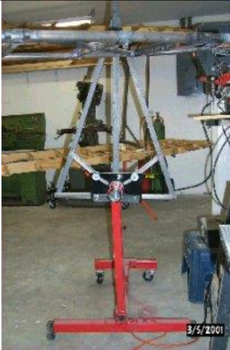
Rear car engine stand, looking from behind (not currently attached to fuselage). The Triangle portion attaches to the hinges of the vertical tail. – see the additional bracket required.
