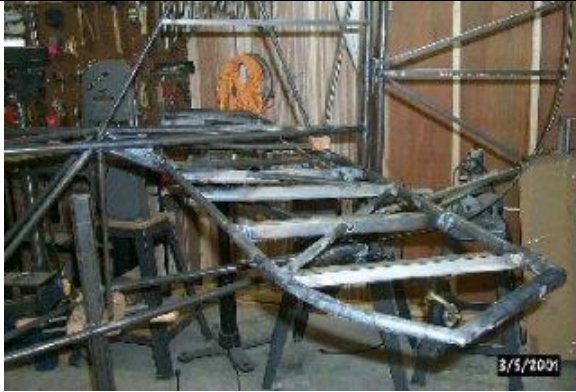
Horizontal stabilizer (without elevator) installed
