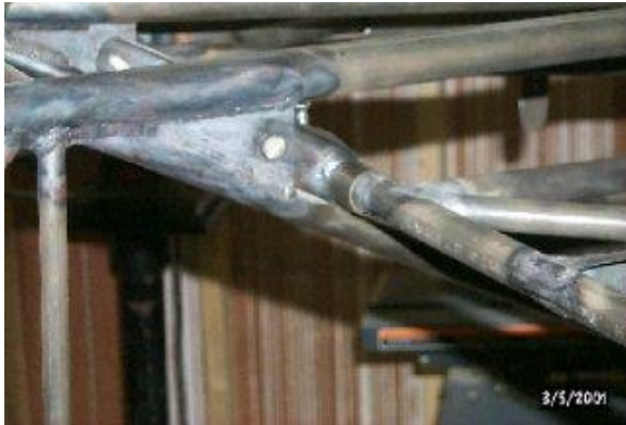
Horizontal stabilizer leading edge attachment
