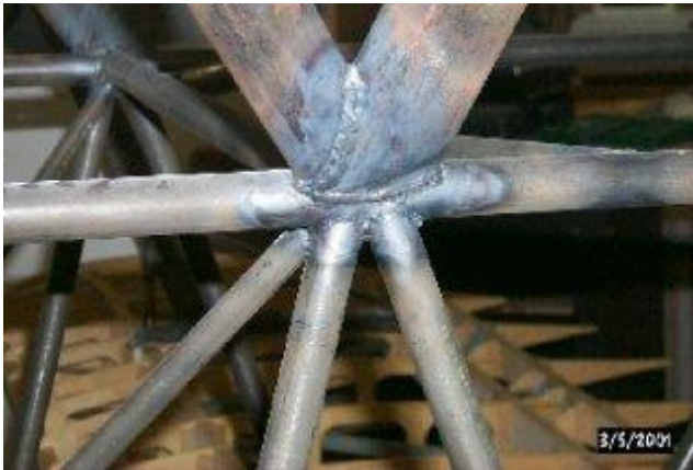
Front of aircraft, looking left side to right side – left rear cabane attachment point
