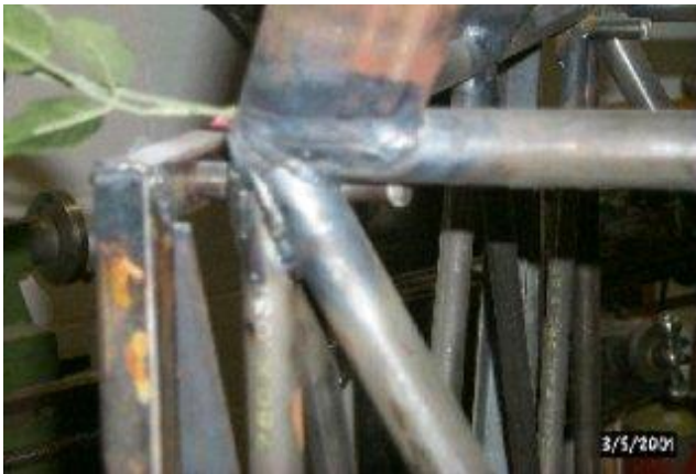
Front of aircraft, looking left side to right side – left front cabane attachment point to engine mount
