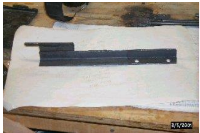
Additional bracket required for attaching the rear engine car stand to the vertical tail.
