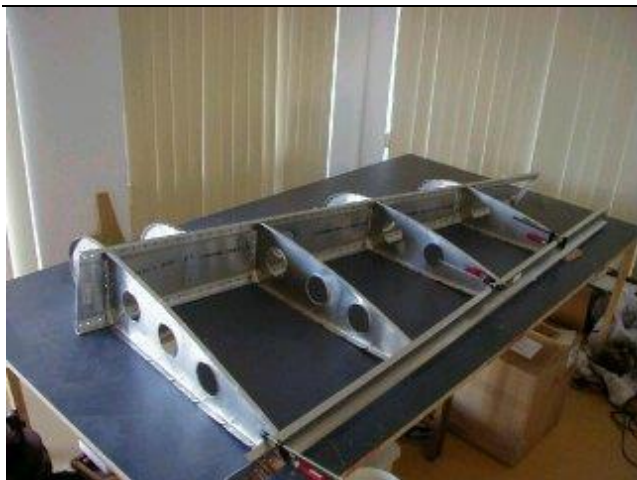
Spars and ribs of one wing panel of Graham's Zodiac
