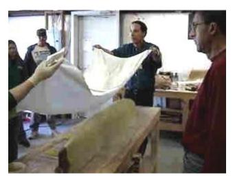
The Master directs the application of the first layer of fiberglass cloth
