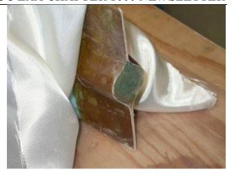
Modeling clay was packed into the aft position light cavity to keep resin out of the screw holes and keep it easy to dig out the foam underneath
