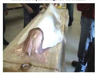
The breather applied over the perf ply. The breather material is essentially the same as batting used in making quilts. Its purpose is to provide an air path between the perf ply and the plastic bag and to absorb the excess resin
