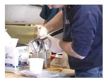
Note the Professor's technique. By pouring the resin in this fashion, more of it goes in the cup and less ends up on the outside of the can
