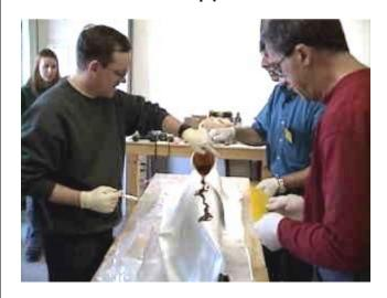
Applying the initial slug of resin
