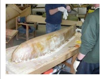
The peel ply is sliced as required and squeegeed into the resin. No resin is added, but the extra resin starts to wick up through the peel ply
