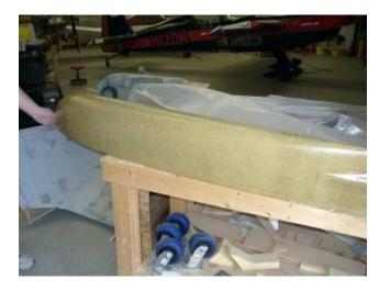
Surface of the wing tip after removing the peel ply and associated bagging materials
