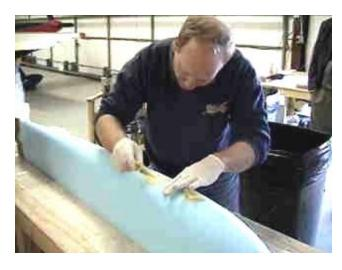
Professor Waldo spreads the peanut butter consistency micro into the divots at the end of the tips. Because the microballoons are filled with air, this mixture is much lighter than epoxy resin alone
