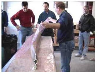
With the "part" resting on one side of the vacuum bag, Professor Waldo applies the perforated release sheet. This plastic sheet has small holes in it to allow the excess resin to pass through into the breather
