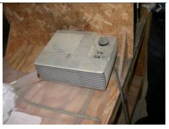
The heat source, an electric space heater specially modified by Waldo to allow it to run at higher temperatures without cutting out
