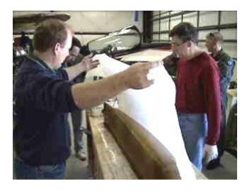
The peel ply is applied. This Polyester (Dacron) fabric has a very low peel strength with the epoxy, allowing the vacuum bagging materials to be separated after the epoxy has cured
