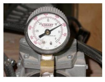
Pressure gauge on the Suckenator, showing about 8.5 psig vacuum
