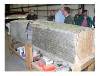
Preparing the heat tent. With the ambient temperature hovering around 59° F (15° C), the epoxy does not flow as well (higher viscosity) and takes longer to cure. This simple heat tent fixes both problems
