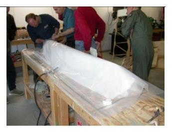
The bag is wrapped around the alien, and the top sheet is carefully pushed down into the sealing tape
