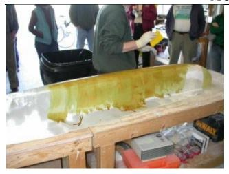
Spreading the resin on the first layer of cloth
