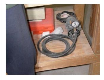
The vacuum pump, aka "Suckenator," stands by ready to remove the excess air. A bleed valve allows setting the vacuum pressure drawn
