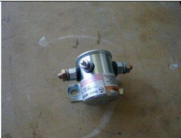
Here we see the offending solenoid as it looked after removal from the aircraft.
