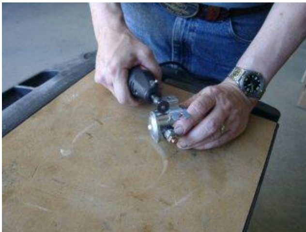
With the skill of a trained surgeon, the steady hands of the Kommandant wield a Project Police Scalpel (a Dremel Moto-tool type device fitted with a fiberglass cutting wheel) to make several cuts through the cap on the solenoid. It's a lot easier to do this when you know that you won't have to reassemble the parts later.
