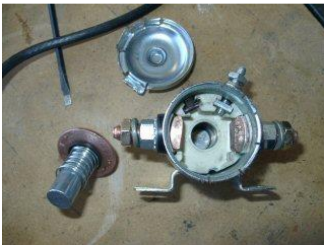
The innards after peeling back the flanges on the cap. The cap is at the top of the picture. Note that the contacts on either side of the inside of the solenoid show noticeable pitting. The plunger (left side) is pulled down by an
