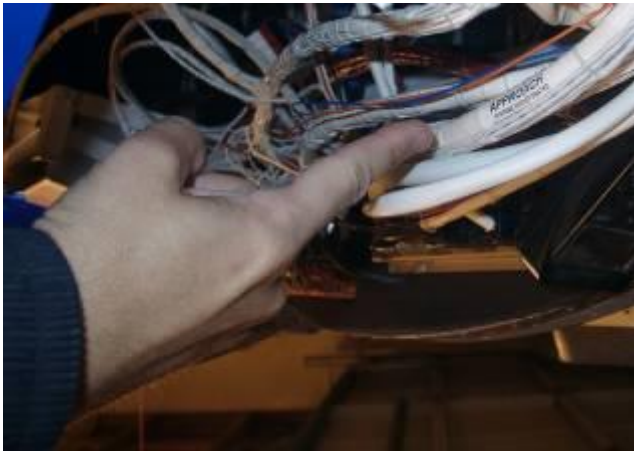
The ASI folks were nice enough to label their cables, but Opus installed them such that we had to turn the airplane upside down to read them!
