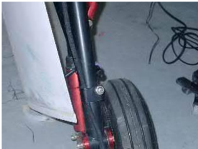
Lipstick camera just above the right main wheel. This sends a picture to the display in the cockpit to reduce the amount of S-turns required to taxi. Seems Jon didn't design a hole through the engine compartment to see where he was going on the ground.
