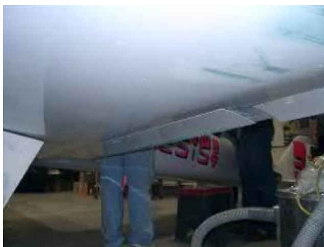
Split flaps (left) and aileron (right). The flaps are the only drag device on the airframe and are rather necessary to be able to slow down for the approach.
