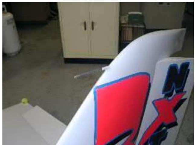
The Pitot tube that helps Jon determine how fast he is zorching across the desert
