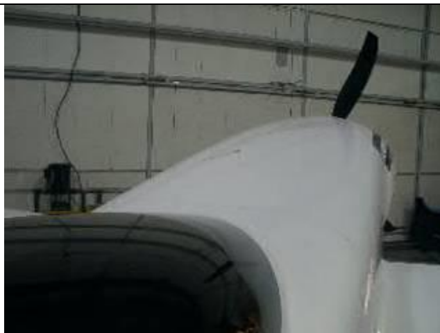
Jon's High-Tech Slip-Skid Indicator—what glider pilots call a "Yaw String" taped to the skin in front of the pilot. He reports it works very well and is very reliable, at least as long as the tape holds. Of course, he is using the highly sensitive pink yarn.
