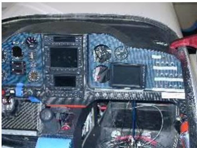
Right hand side of the instrument panel. Center stack has enough Garmin hardware to make the Kommandant weep with jealousy. Control stick is between the seats. Display screen on the right hand side is connected to a camera on the right main landing gear.
