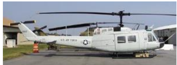
HU-1H With Longer Aft Fuselage of UH-1D
