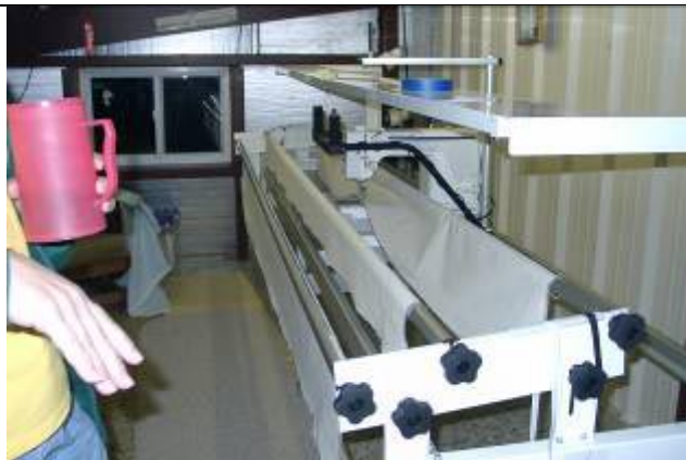
Gail's super-cosmic laser guided sewing machine. The fabric remains stationary while the sewing machine can be manually moved fore and aft and side-to-side. The position of the needle is shown by a laser on the upper shelf, which can be used to trace patterns. Gail says this setup is for quilting, but we not so sure there isn't some classified project going on here...
