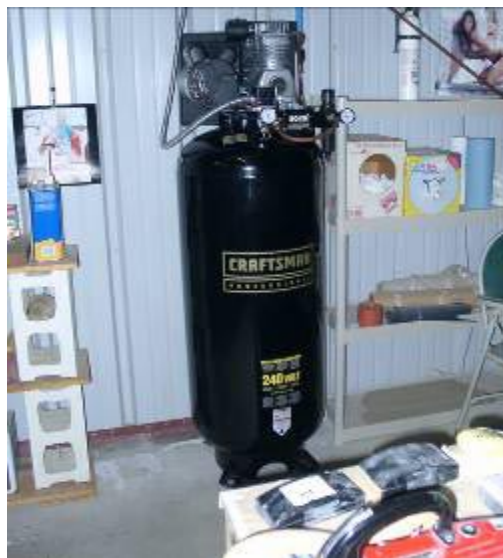
One of Opie's recent projects was installation of this mega-mongo air compressor and air distribution lines. He'll need that capacity to run the air powered sander to prepare the Glasair for finishing
