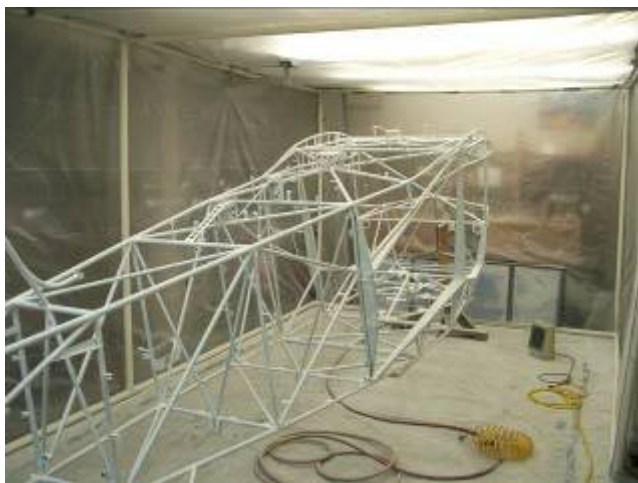
Erbman's fuselage after priming (taken on 4 Dec 2005)
