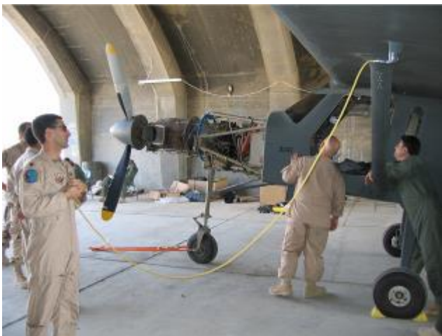
Pitot-Static leak testing the high-tech way. Obviously Erbman has trained him well
