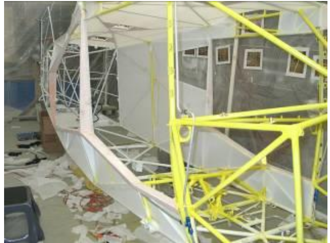
Back to White and Yellow with application of interior fabric, 19 Mar 06
