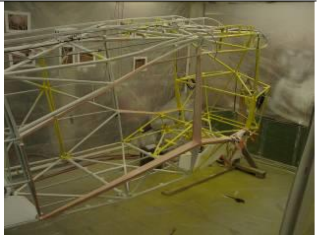
Yellow and White...and...uh...(manly) Pink. Poly Brush painted onto large areas of fabric that would be in contact with the fabric to prevent pinholes
