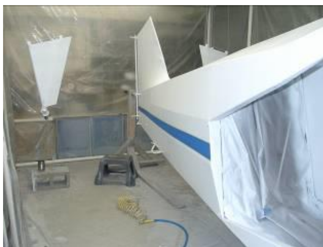
White and Blue—future red stripe masked off with Fine Line and blue painter's masking tape, 3 Jul 06
