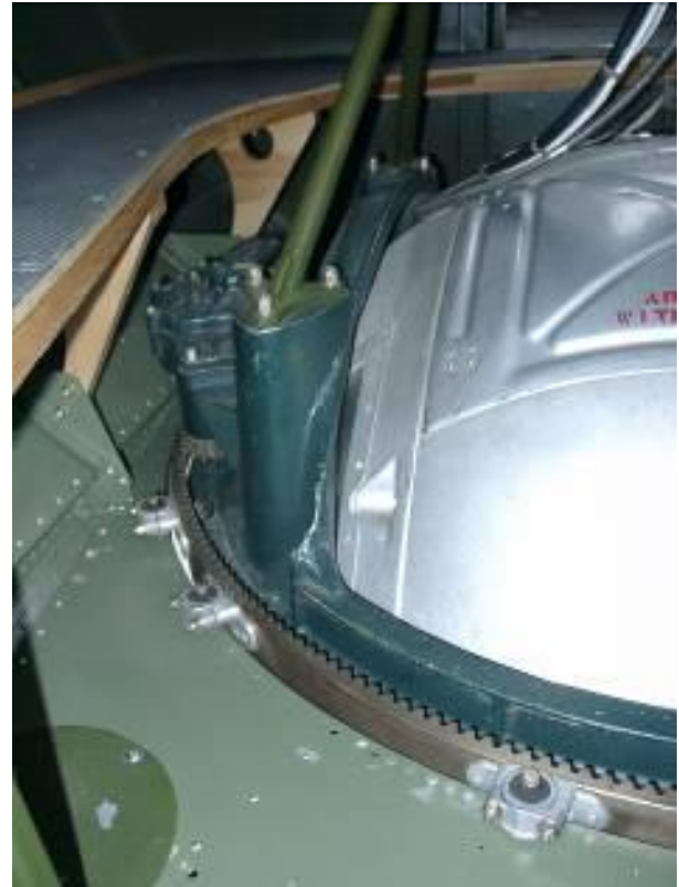
Ring gear and pinion (left side) for rotating ball turret in azimuth
