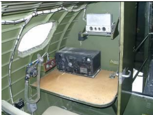
ADF unit, with oxygen regulator on left sidewall
