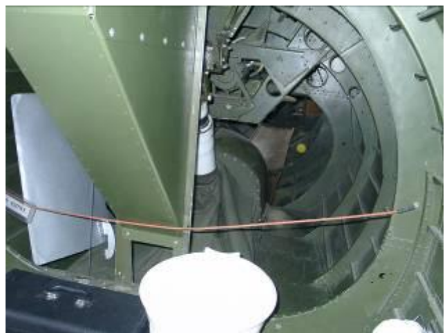
Tail wheel assembly. This way back to the tail gunner position.
