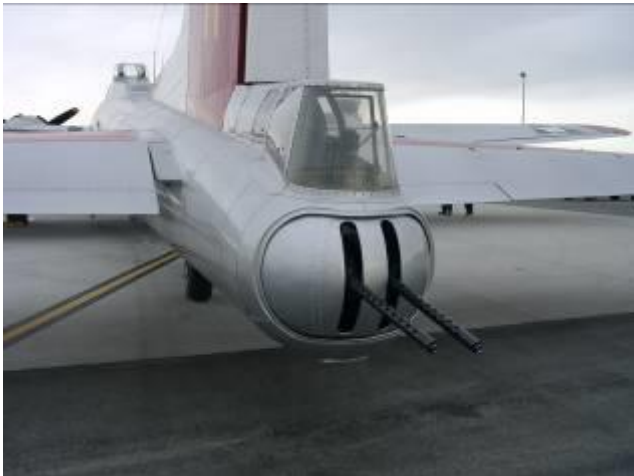
Tail gunner position with larger windows found on late model B-17Gs
