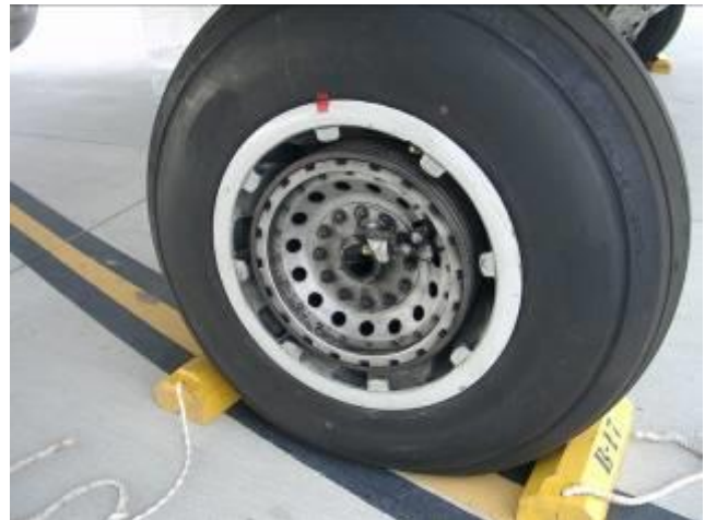
Old fashioned hydraulic expander brakes, built well before the clearly superior disk brakes were developed
