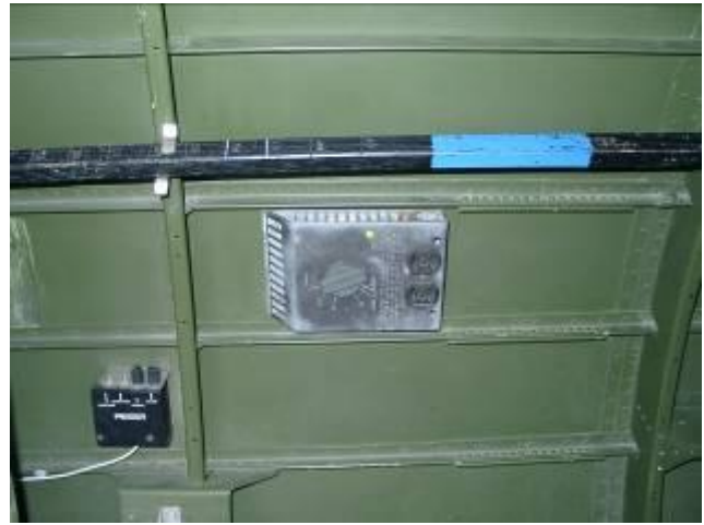
Outlet for electrically heated flying suit. Note stringer splices to the right.
