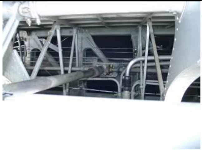
One of five flap actuation jackscrews. Note truss wing rib construction, truss rear spar construction, and large number of stringers on the upper (compression) wing skin
