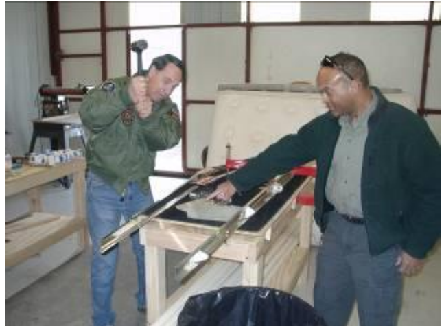
Vice Kommandant Knife Gennuso and Brian Martinez demonstrate their experimental rivet driving technique – no air compressor required
