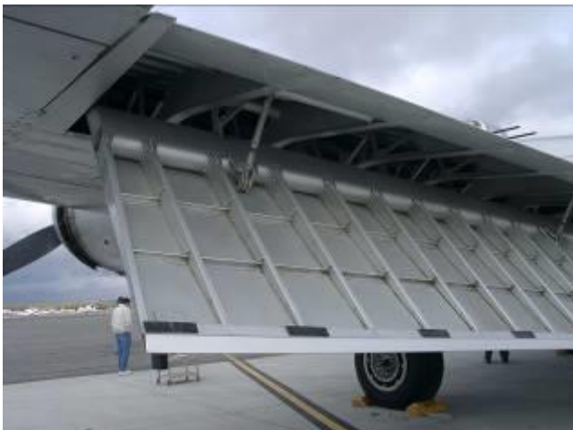
View showing hinge rods that force the flap down as the jackscrews push aft
