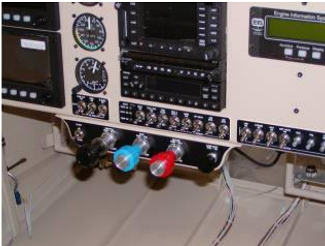
Jim did his switch placards the same way that Erbman did, which was the same way that Opus did, using engraved aluminum strip from http://frontpanelexpress.com/ , which happens to be just down the road from him in Seattle
