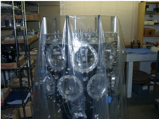
Not all V-12s have 12 cylinders or even arrange them in a "V" configuration. This is the core of a Bristol Centaurus engine. This was a British radial that used sleeve valves instead of poppet valves. Because of its complexity and limited production, many fliers of Centaurus-powered aircraft have replaced their Centaurus engines with American Pratt&Whitney or Wright radials.
