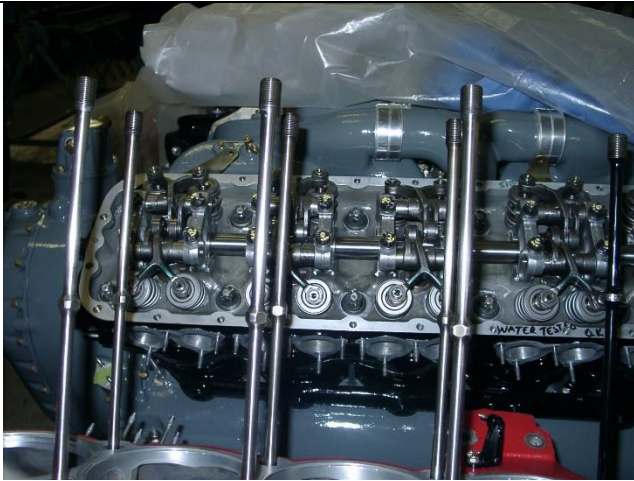
The Allison uses a camshaft under roller cam followers. Only one cam lobe is used per rocker arm. Each rocker arm actuates two valves.
