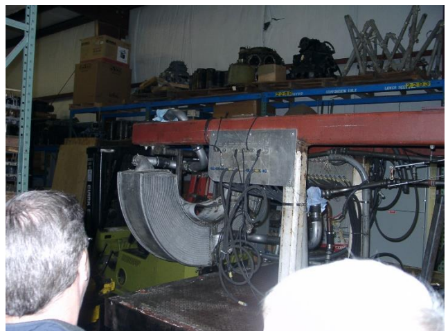
Part of the engine ground test rig mounted on the bed of a large truck. Using a truck allows the engine to be built up out of the weather, then moved outside when conditions are right for testing.
