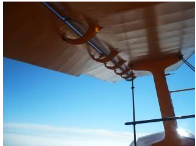
Extended flap and drooped aileron on the top wing
