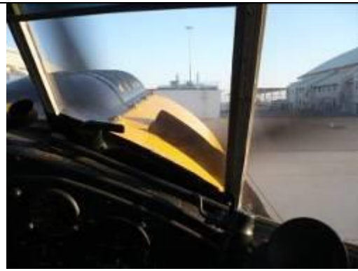
Direct-indicating cowl flap as seen from copilot's seat
