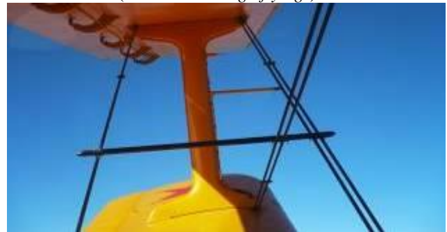
Drag producing hinges, wires, and javelin. Pitot-static boom and temperature probe extend forward from the interplane I-strut
