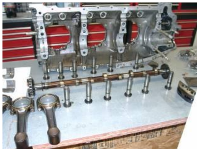
Crankcase half, camshaft, lifters, and other parts
