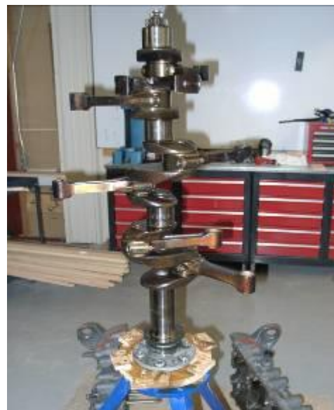
Crankshaft before removing connecting rods and counterweights (which are actually dampers)
