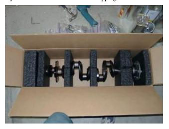
The fine folks at AEA inspected the parts and decided on a course of action. The crankshaft main journals were ground and polished to .006 undersize. The crank journals were ground and polished to .003 undersize, just enough to remove any damage. After machining the crankshaft was nitrided, a casehardening technique using nitrogen at elevated temperatures.
