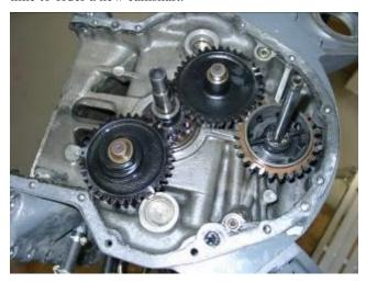
A fun little note in the overhaul manual stated that anytime the camshaft was reground and rehardened or simply replaced \*ALL\* of the lifter bodies must be replaced. Fortunately, these are sold in a kit with the new camshaft.
