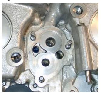
The worst was the oil pump drive shaft, which drives the gear with two flats. These flats were rounded off so bad (like when you round off a stuck nut using the wrong wrench) that only half of the flat was still flat, and you could poke a welding rod in the gap that was left. I ordered up new oil pump gears (they only come as a set) of the proper type, a new housing, and a new drive shaft. That is to say, a new oil pump.
