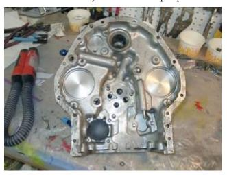
Inspection of the oil pump was like a "Little Shop of Horrors." The drive gear looked brand new and was of the proper type according to the famous Lycoming Oil Pump AD. That's where the good news ended. The driven gear was an old aluminum gear, a combination originally allowed but now required to be replaced "at the next overhaul" by the AD. Inspection of the oil pump housing and the accessory housing showed excessive scoring where the gears had rubbed on the sides, as seen here.
