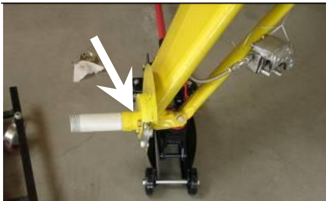
Axle with wheel removed and brake caliper tied up out of the way. The wheel bearings rest on the white part of the axle. The torch was applied and the axle bent at the point shown by the arrow.
