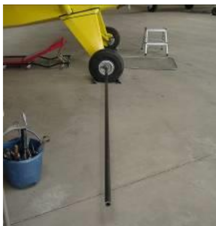
The Bar to Apply Torque for the Purpose of Increasing Stress and Strain (BATPISS), an 8 foot long section of 1-1/4 x 0.120 4130 tube that slipped into the axle.
