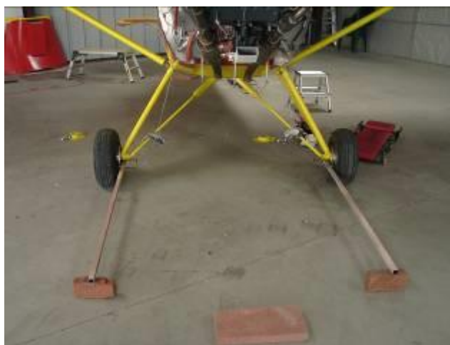
To measure the toe-in, square tubes were clamped to the brake disks. Measurements were taken against a centerline marked by plumb lines from the tailwheel spring and crankshaft.
