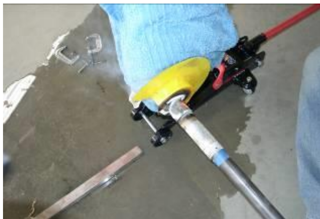
Axle after bending—note red glow. Towel over fabric gear leg is dripping wet to protect the fabric
