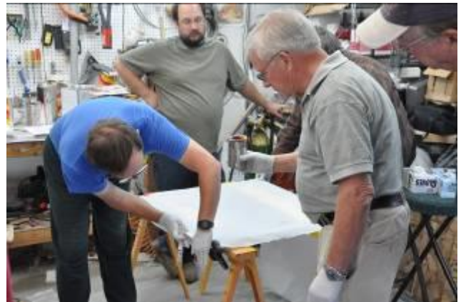
The Poly Prof expertly demonstrates the "brush and smash" method of fabric cementing as Hellmuth holds the well-used Poly Tak can
