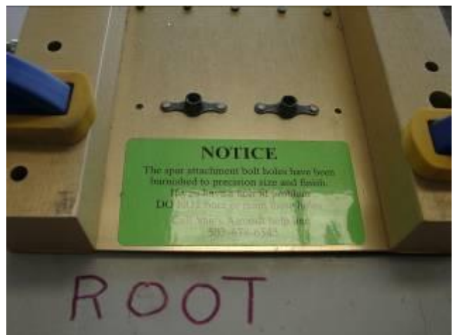
It's entertaining when the kit manufacturer has to put notes, warnings, and cautions directly on the parts
