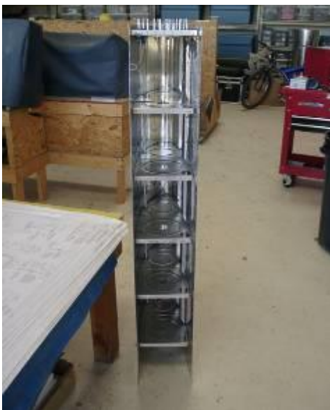
One of the fuel tanks. As it is, this will never hold water, or fuel for that matter. We suggested that it needs another side.
