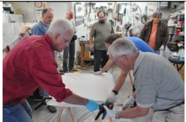
Clamping the fabric into place prior to cementing around the frames
