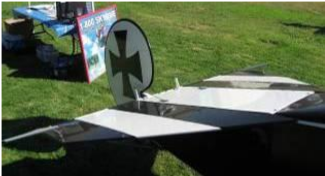
Tail of the triplane, with the very flat and rather large horizontal tail and the very small rudder with no vertical stabilizer. Apparently Reinhold Platz hadn't figured out that directional stability thing yet.
