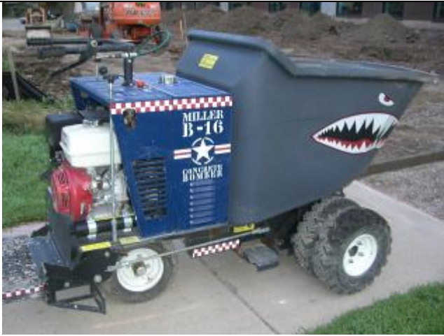
Stormy was fascinated by this motorized concrete dumper, used to carry away the rubble.
