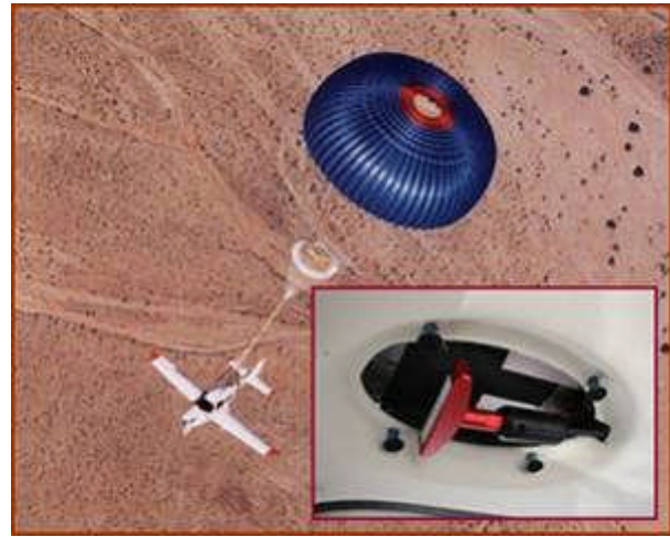
Ballistic recovery system used on Cirrus airplanes. Inset shows the deployment handle.
