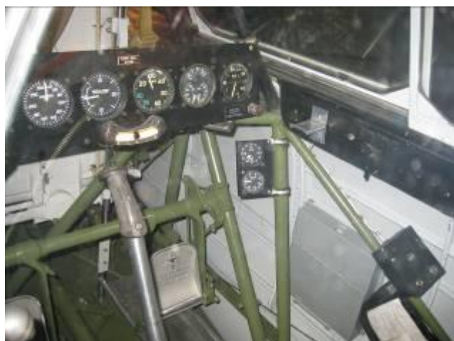
Rear cockpit with greatly reduced instrument panel
