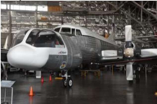
The Calspan Total In-Flight Simulator (TIFS), NC-131/N793VS. You'll find this aircraft in Aldrich, Erb, and Dodson's logbook in the Advanced Systems Test and Training Aircraft (ASTTA) configuration
