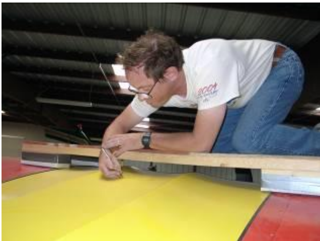
On the "Bridge To Nowhere" cutting the fabric to make room for the new mounting screws
