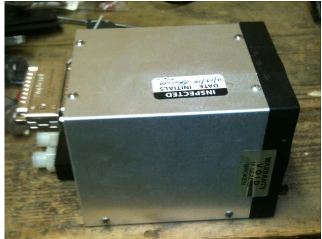
New metal case with RF filter connector mounted to DB25 connector
