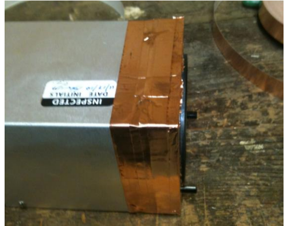
Copper tape bridging the gap between the metal case and instrument panel
