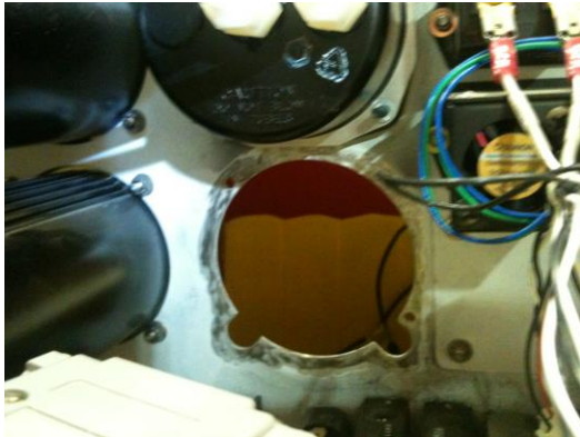
Autopilot mounting hole with non-conductive paint removed
