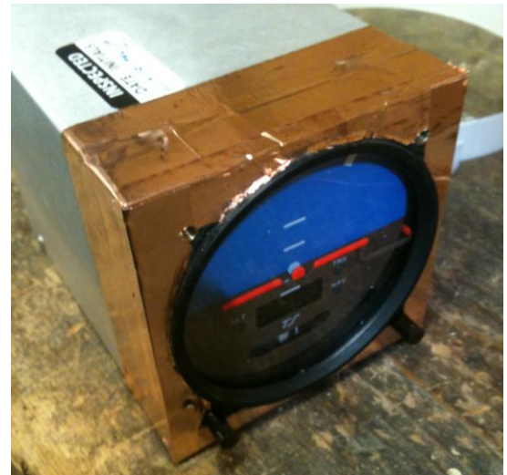
Copper tape wrapped onto front of case to connect with instrument panel
