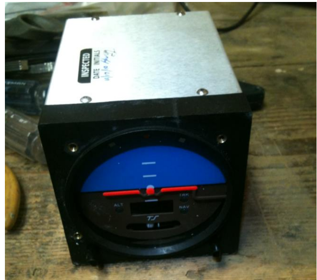
Plastic faceplate which gave an entry path for RF interference
