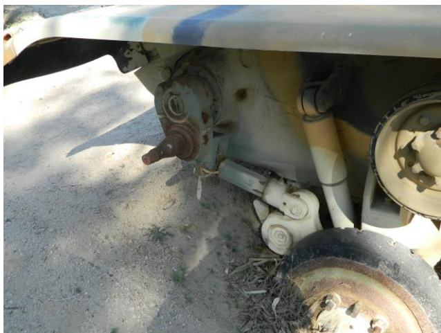
At the other end we found what appears to be the track tensioning mechanism
