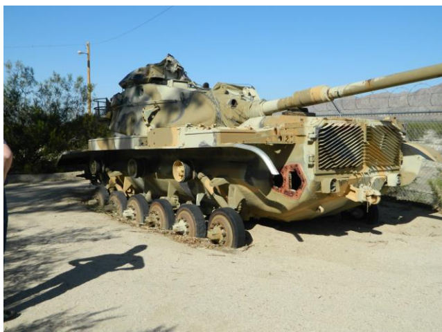
This trackless wonder seems to have sunk into the dirt until the hull is floating. At the near end the drive shaft and gear seems to be missing.
