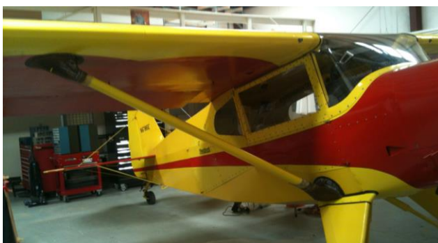
Right side fairings installed. The upper fairing is screwed into the wing. The lower fairing is clamped around sandpaper on the strut.
