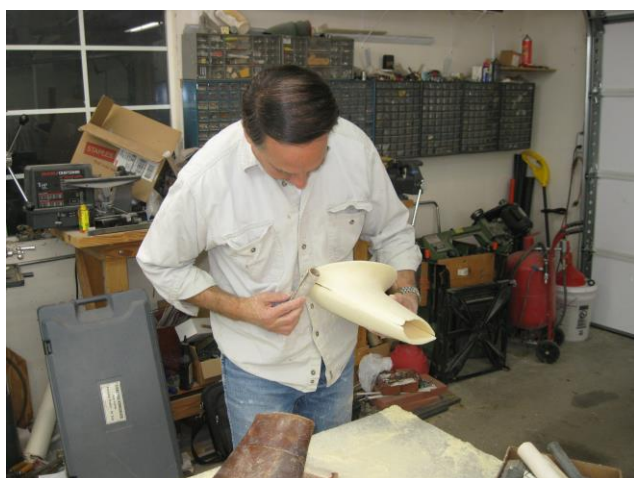
Knife carves the lower strut fairing with a PVC pipe and a piece of coarse sandpaper. Note the very fragile and very thin foam section around the strut. It's amazing that we never broke it.
