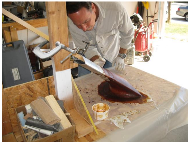
A special fixture was needed to glass up the lower fairing using the strut cut-offs
