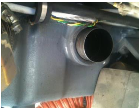
The loose intake tube in the oil pan
