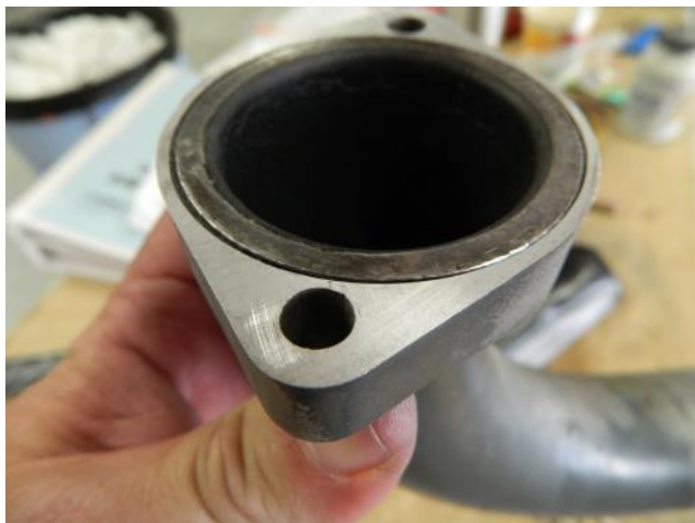
The flange after sanding it down level with the intake pipe
