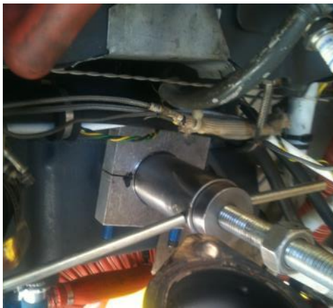
Beading tool inserted into tube
