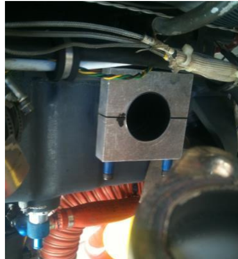
Clamp to hold the tube in place while swaging
