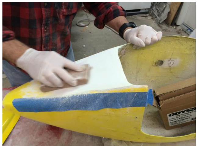
After the filler has cured, it is sanded to the final shape. Some builders (like Knife) really enjoy this step, others (like me) not so much
