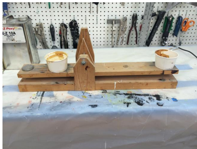
Knife's magic balance, which mixes 100/44 by weight. This balance measured all parts on Knife's Pulsar and Erbman's Combat Bearhawk
