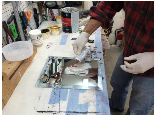
Mixing the body filler (“Bondo”). The mixture is a “golf ball” of filler to a “pea” of hardener. Mixing on a thick piece of glass; in this case, a cheap mirror
