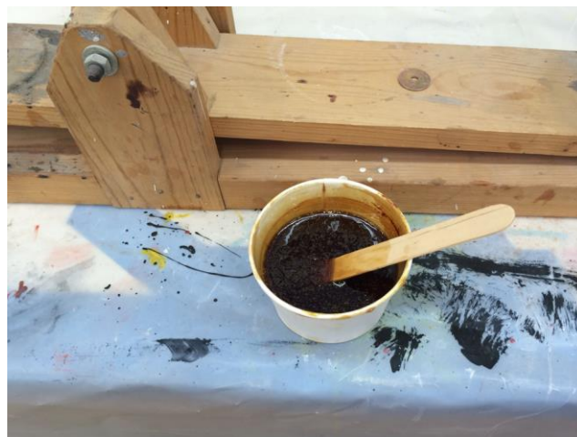
The epoxy after mixing. When new, it mixes up a much lighter color. With age the Part B absorbs moisture from the air and gets darker
