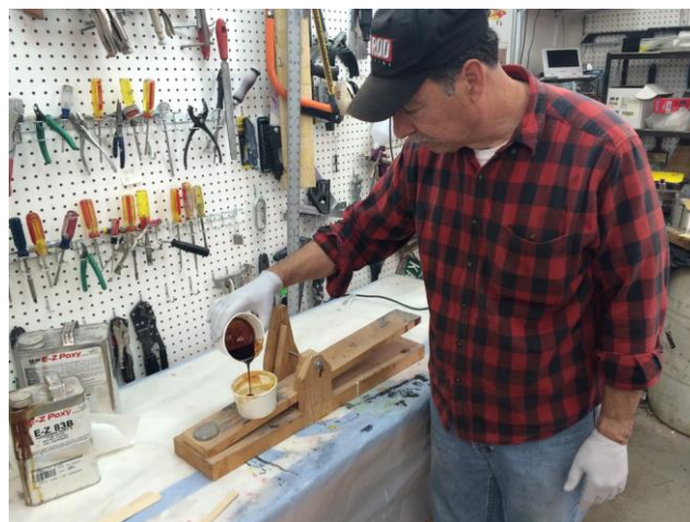
Knife mixing the epoxy, which now gets stirred for three minutes
