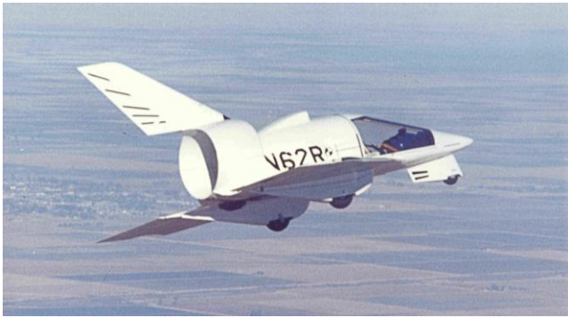
71-X in flight photo over the Holtville, California farm area. Note the drag chute packet tucked under the duct
