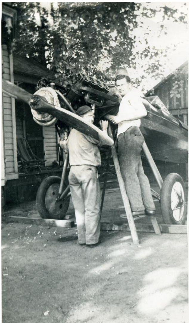
My Dad, Harley (on ladder with ever-present cigarette) and my great-uncle Earl Bavis deep in the process of overhauling the tank engine. Note the lack of braking equipment on the big wheels
