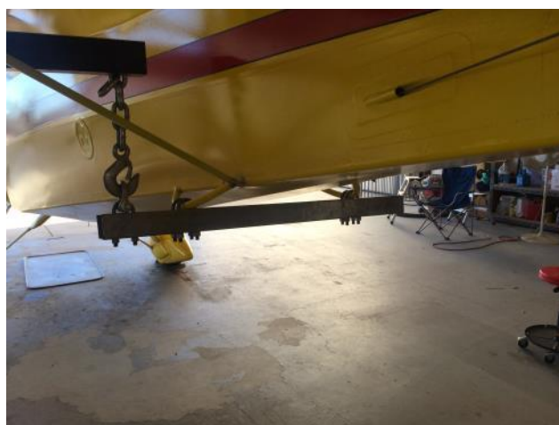
Close-up of lifting fixture attached to fuselage handles.
