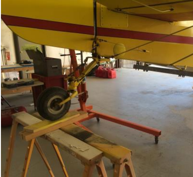
Tailwheel supported on sawhorses and blocks
