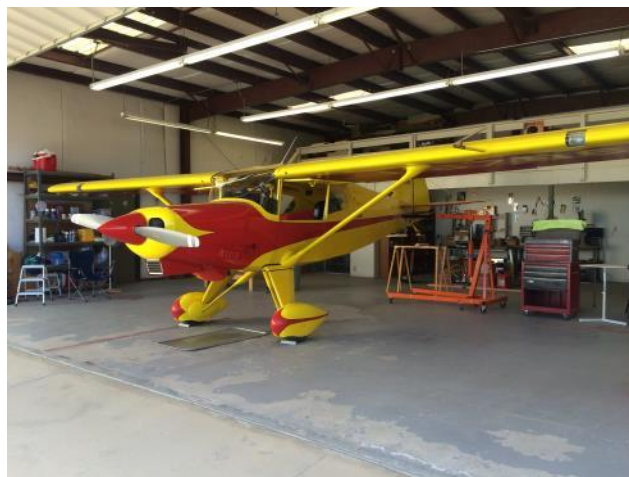
Tail raised to fuselage level position (nominally flight attitude)
