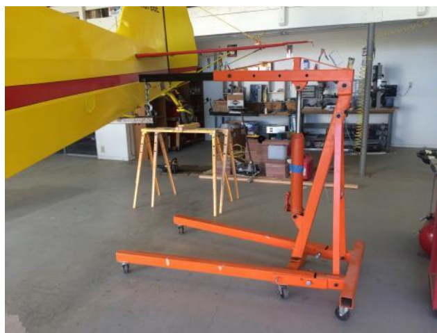
Shop crane to do the heavy lifting
