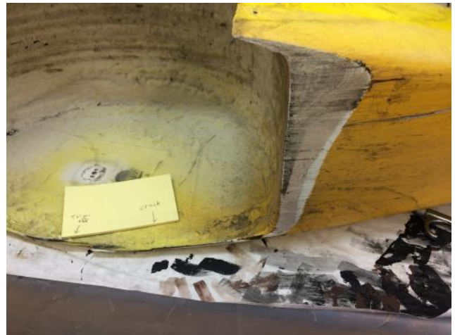
Wheel pant damage. Post-it points to a small break and a crack. Bottom side shows a little wear
