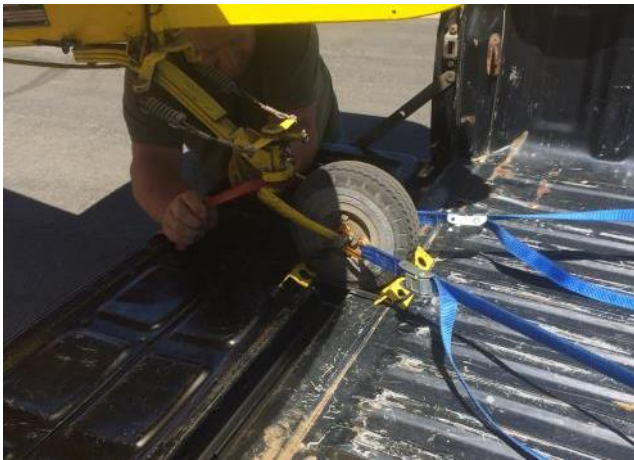
Tailwheel chocked and strapped into position three ways
