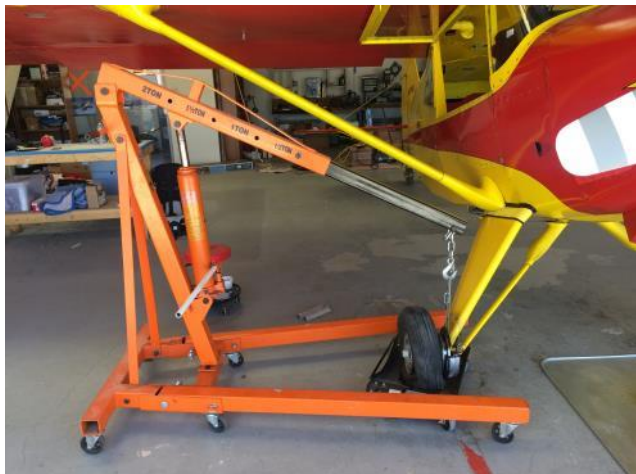
Using the shop crane and a cable to lift the sore foot off of the car dolly
