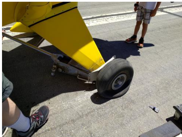
Wheel pant removed. Tire is sad.
