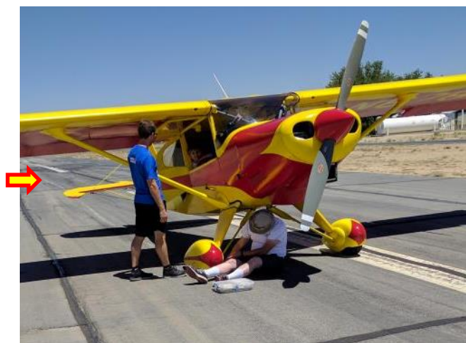
Same picture, zoomed in. Arrow shows start of skid mark where the wheel pant touched the runway. The skid mark is only about 130 feet long.
