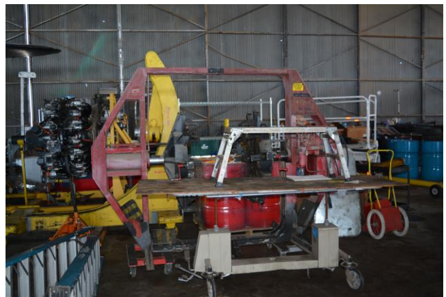
The most entertaining find was this rust-brown fixture, which is a bead breaker for B-29 size tires
