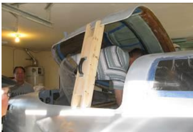
The solution to the overgrown gas spring is the over-engineered canopy prop. It is beautifully fabricated with a fancy handle, but we suspect this is not flight-weight hardware
