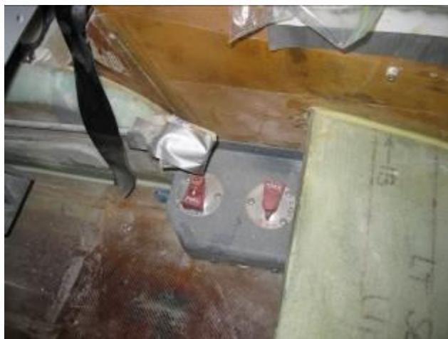
Two engines need two fuel selectors, cleverly arranged fore and aft
