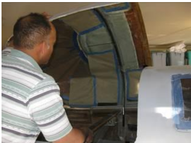
The canopy is not held up by the disconnected gas strut. Brian says the one installed here is too strong and it is difficult to close the canopy.
