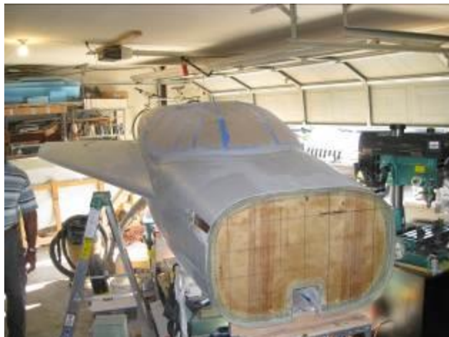
The forward firewall. One engine goes here. Also visible are the pivot for the retractable nose gear and the slot for the canard spar.
