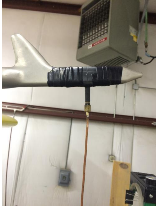
First iteration of Pitot-static tube adapter
