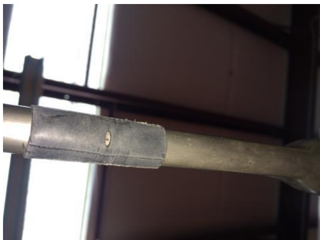
Inner tube stretched over Pitot-static tube, aligned over static port
