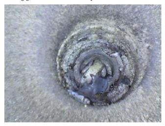
That's the lower spark plug, with a whole bunch of **krap** on it. Lead fouling, to be specific. I've never seen so much fouling on any plug on this engine.
