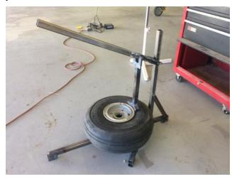
So how well does it work? After deflating the tire by removing the valve stem core, an easy push on the handle drove the bead right down with very little effort.
