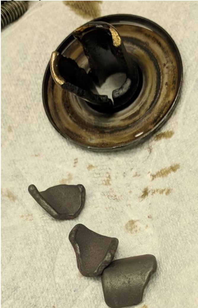
Aren't these all supposed to be one piece? (The three pieces on the bottom fell out of the heat exchanger)
