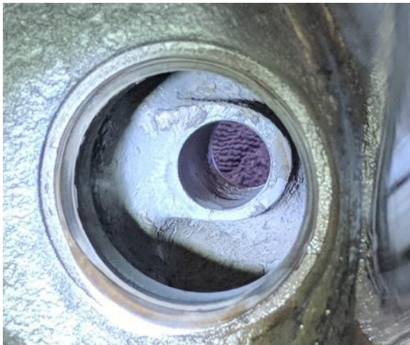
Badly worn valve seat – and missing guide
