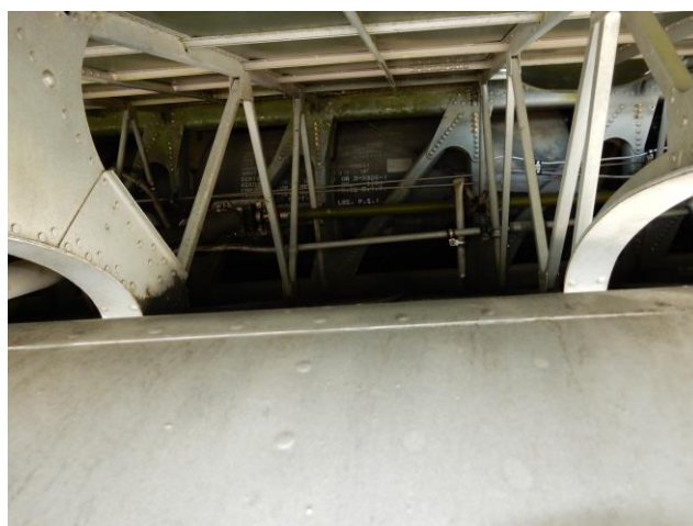
Fuel tank view through the Fowler flap on the left. Flaps and landing gear are electric.
