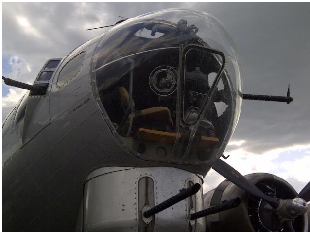
Nose gun configuration. This is a typical set up for later models. Side guns are the cheek stations. The chin turret is non op. Another project.
