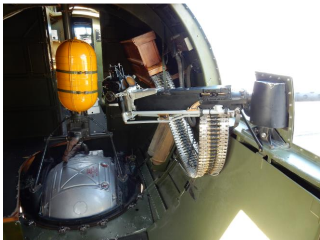
Waist gun with the "whole nine yards" mounted behind. Oxygen tank for the crew is mid fuselage and the top of the ball turret is below.
