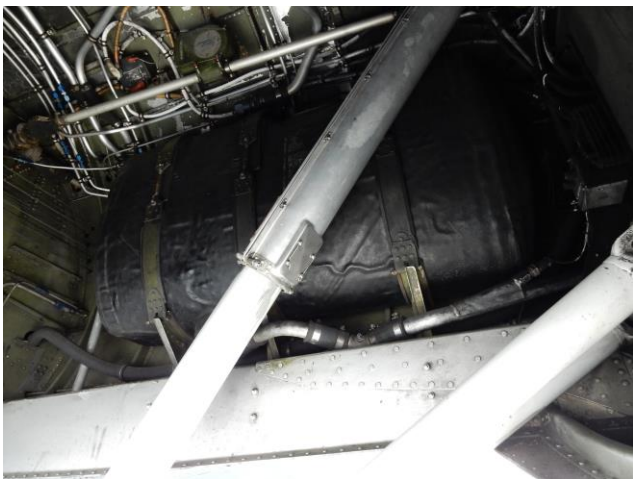
Engine oil tank. Aft of the inboard engine and viewed through the wheel well. One of the mechanics told me they went through gallons on a typical tour flying day.
