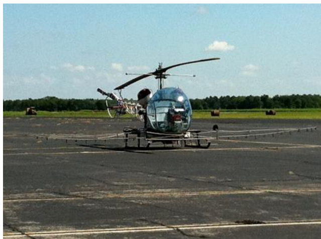
Spray bar equipped Bell Model 47 as seen at Pine Bluff Airport AR (KPBF) on 18 July 2011
