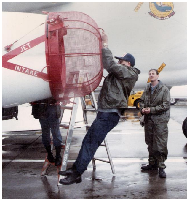
Lee Erb conducting a carefully planned ground test on the security of an intake screen on an A-3 at Alameda Naval Air Station
