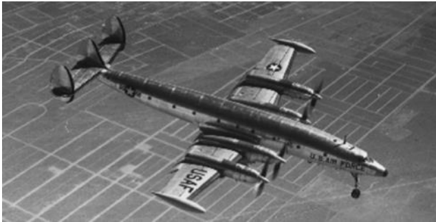
YC-121F with P&W YT-34-P-12A turboprops
