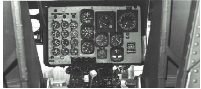
H-21C Pilot and FTE station, with sensitive tachometer, altimeter, and manifold pressure
