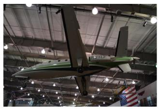
The Y-tail was unique. As is common with pusher aircraft, the ventral vertical tail prevents prop strikes with the ground by smacking the ground first. This vertical fin carried the only rudder. Unlike the Bonanza, the surfaces on the upper "V" tail were only elevators. There was no pitch/yaw mixing in the tail. Quiz question: Which rudder is needed on takeoff and climb? Prop rotation is still clockwise viewed from rear.
