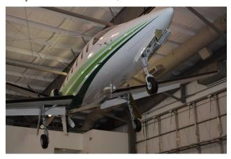
In the 1970s, composite construction was all the rage. The Lear Fan was built from mostly composites, and much like the Beechcraft Starship, this led to certification problems. Since composites were "new" the FAA didn't have the experience to know how much they could trust them. This led to larger and larger factors of safety, which meant that the airplane got heavier and heavier, which is never good. Structural problems were discovered during pressurization of the fuselage.
