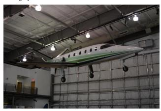
At first glance, the aircraft appears to have a small turbojet engine on either side of the aft fuselage. These are really just pods that serve as the intake and exhaust for two PT6 turboprop engines mounted inside the fuselage. These
