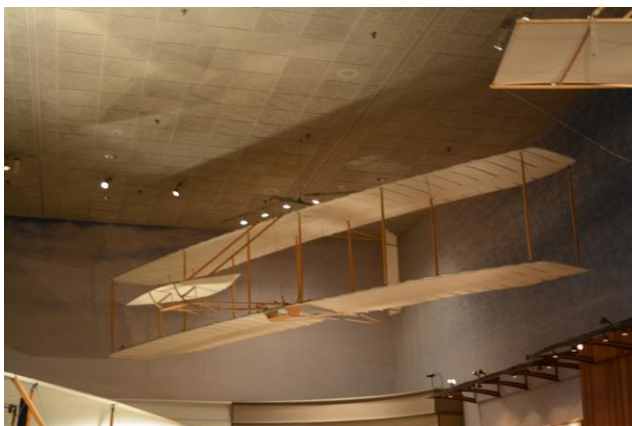
Second glider flown at Kitty Hawk. This one shows the higher aspect ratio require and also the addition of a rudder for directional control and stability
