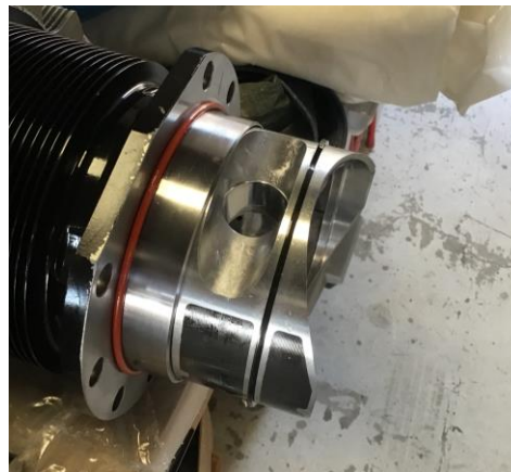
Rings compressed and piston inserted into cylinder
