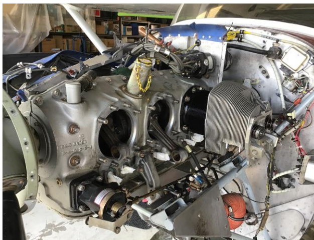
One left side cylinder installed
