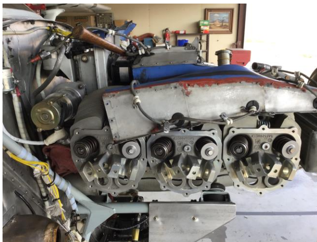
Right side cylinders awaiting rocker arms
