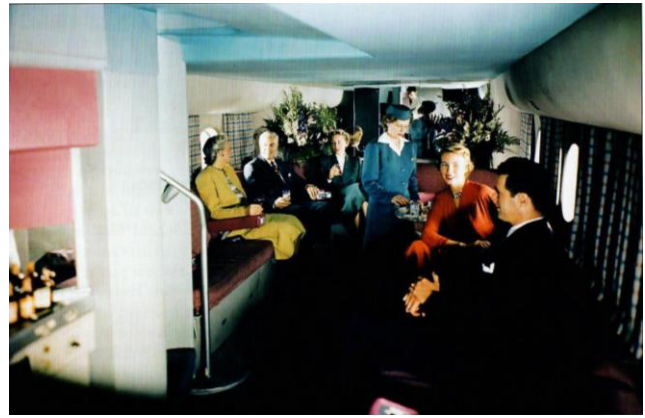
Looking rearward in the Stratocruiser lounge. The bottom floor between the seats is actually the curved underside of the fuselage. 3
