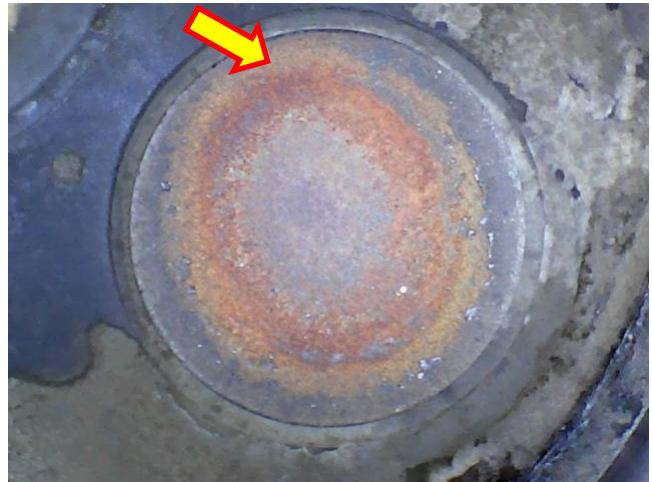
Cylinder #1 in 2018. Arrow shows where burn marks are getting less circular and working toward the edge
