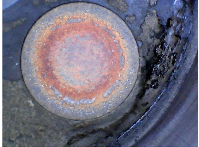
What an exhaust valve should look like, the symmetric “burnt pizza” (Cylinder #2, 2018)
