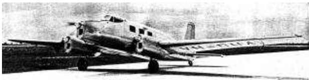
The de Havilland DHA-3 Drover Commercial Monoplane (three 140 h.p. D.H. Gipsy Major 10 engines)
