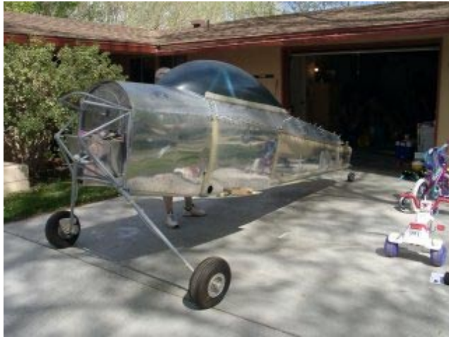
RV-4 fuselage with canopy installed
