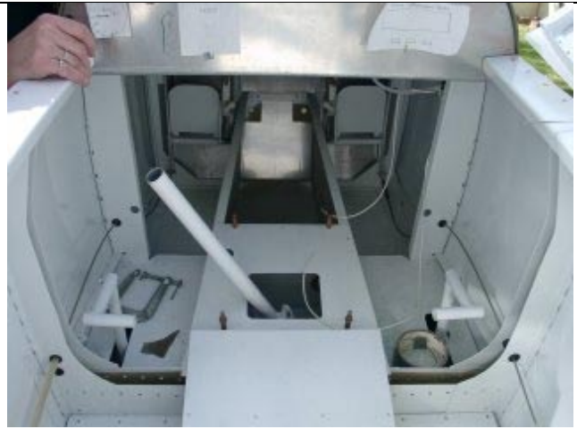
Dave is installing rear seat rudder pedals. These connect to the front seat rudder pedals by simple push-pull rods.
